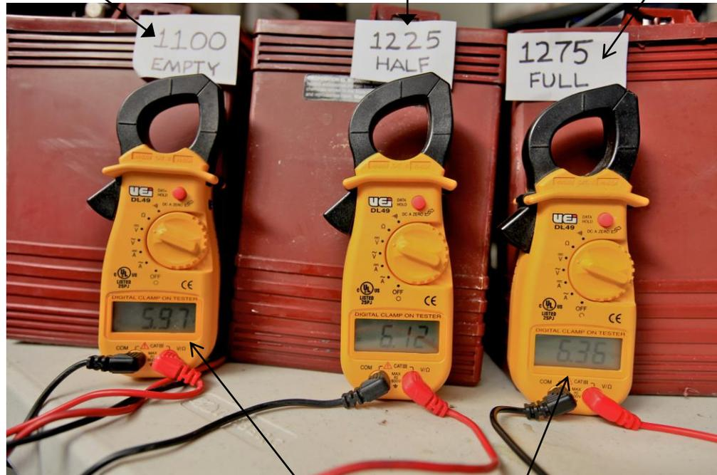
Big difference in gravity level of 175 points. Easy to find dead battery with a hydrometer over a volt meter.
