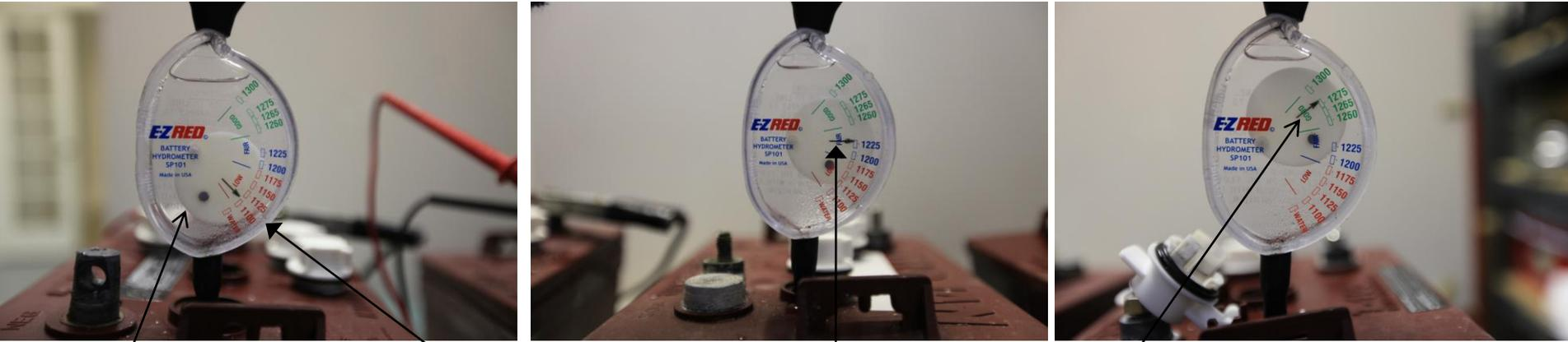
Use a hydrometer to get an accurate indication of how much charge is in the battery
